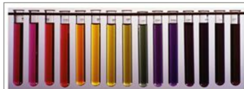
▲ Universal indicator turns orange in vinegar. It turns red in stomach acid.
