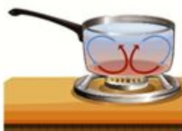
▲ A convection current in a saucepan of water heats all of the water up.
